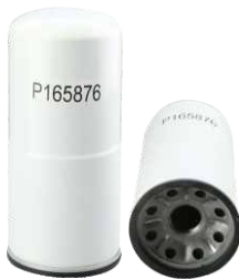
KFH 0727 Outer Diameter [mm]:121,4 Seal Diameter [mm]:128 Thread Size:1 1/2-16 UN Height [mm]:270,7 P165876 H306W 177356A1 1329214C1 A177605 HF28929 Application: DONALDSON
