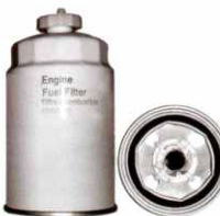
KFF 0666 Largest OD: 85(mm) Overall Height: 163(mm) Thread Size: M16x1.5 OEM: 87800220 NEW HOLLAND: 87800220
