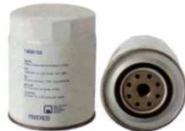
KFO 0662 Largest OD: 108(mm) Overall Height: 145..5(mm) Thread Size: 3/4"-16 OEM: 1909102 IVECO: 1901602, 1907567 PERKINS: 26540215 RENAULT: 5000041045 HENGST: T208W01
