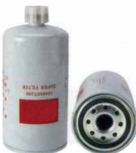
KFF 0458 Largest OD: 94(mm) Overall Height: 201(mm) Thread Size: 1"-14UNF OEM: 16400DT300 FLEETGUARD: FS1212, 16400DT300
