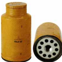
KFF 0351 Largest OD: 108(mm) Overall Height: 180(mm) Thread Size: 1"-14 OEM: 1R-0769 CAT: 1R-0769 FLEETGUARD: FS19843
