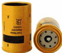
KFF 0353 Largest OD: 94(mm) Overall Height: 138.5(mm) Thread Size: 1"-14 OEM: 1466695 FLEETGUARD: FS19776
