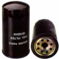
KFF 0655 Largest OD: 92(mm) Overall Height: 176(mm) Thread Size: M24X1.5 OEM: 4616544 HITACHI: 4616544 FLEETGUARD: FF5367
