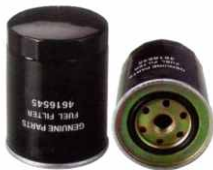
KFF 0654 Largest OD: 92(mm) Overall Height: 125(mm) Thread Size: 3/4"-16 OEM: 4616545 HITACHI: 4616545 FLEETGUARD: FF5108
