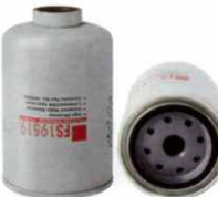
KFF 0461 Largest OD: 94(mm) Overall Height: 145(mm) Thread Size: M20X1.5 OEM: FS19519 FLEETGUARD: FS19519
