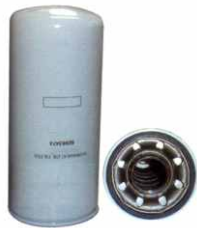
KFH 0659 Largest OD: 118(mm) Overall Height: 260(mm) Thread Size: 1 3/4"-16 OEM: 82983474
