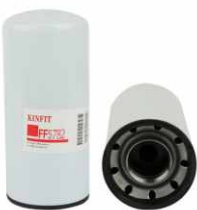
KFF 0457 Height: 266.73 mm Thread Size: 2 1/4-12 UNS-2B Outer Diameter: 118.11 mm OEM: FF5782 2881458
