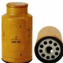
KFF 0352 Largest OD: 108(mm) Overall Height: 180(mm) Thread Size: 1" 14 OEM: 326-1644 CAT: 326-1644,1R0770 FLEETGUARD: FS19820
