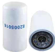
KFH 0660 Largest OD: 136(mm) Overall Height: 246(mm) Thread Size: 1 3/4"-16 OEM: 82005016 NEW HOLLAND: 82005016 81865736 FLEETGUARD: HF28885
