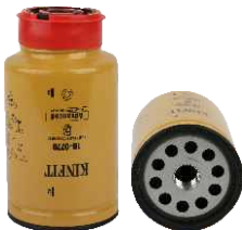
KFF 0348 Largest OD: 108(mm) Overall Height: 180(mm) Thread Size: 1"-14 OEM: 1R-0770 CAT: 1R-0770 FLEETGUARD: FS19820
