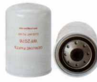
KFW 0472 Largest OD: 94(mm) Overall Height: 135(mm) Thread Size: 11/16"-16 OEM: WF2076 MANN: WA95612 CUMMINS: 3100309
